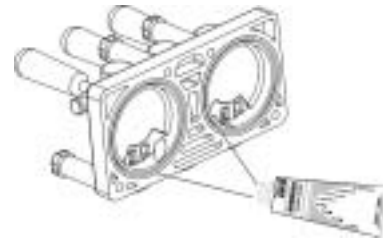
Picture 9: the Discharge door lubrication
